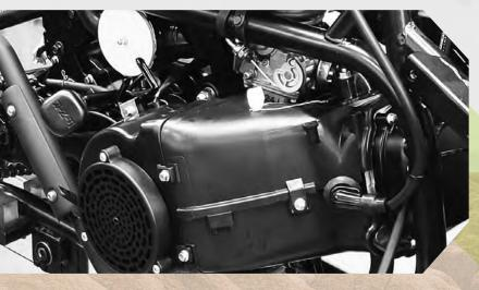
The ATV TITAN 200 comes with 177,3 cm³ liquid-cooled, 4-stroke single engine with power of 9,86 Hp at 7.500 rpm and a maximum torque of 10 Nm at 6.000 rpm.
