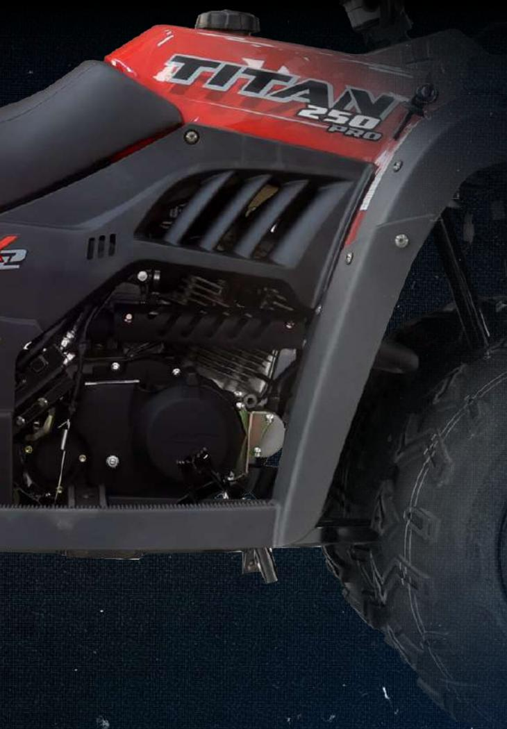
**POTENCIA****14,75 hp @ 5.500 rpm****TORQUE MÁX.****15.5 NM @ 5.500 RPM****MOTOR CON
